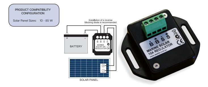
The Sealite Marine Solar Regulator is ideal for marine installations. The regulator acts as an intelligent switch between the battery terminal and the solar panel.
