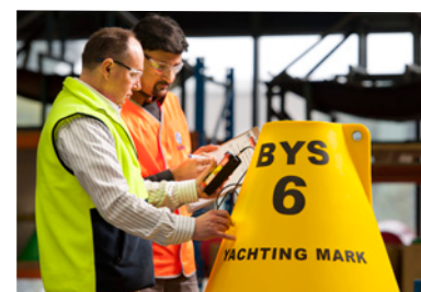
The wall-thickness of each buoy is measured in critical areas by ultrasound
