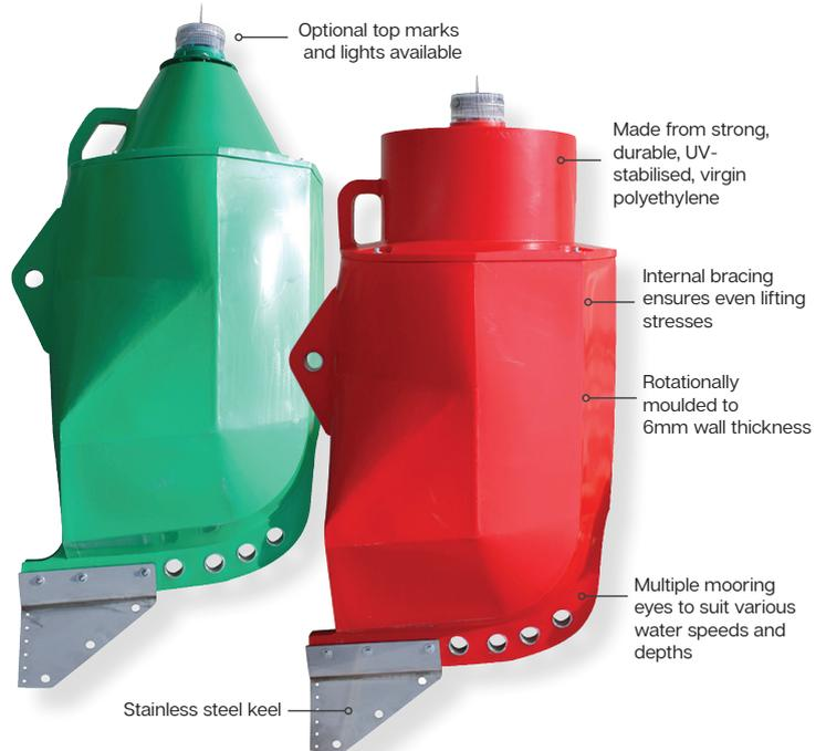
The unique, one piece float section has an internally integrated bow and keel which ensures the buoy remains stable during fast currents. The SL-B750 is rotationally-moulded from UV-stabilised, virgin polyethylene in a range of IALA recommended configurations and colours to ensure clear visibility, and may be fitted with a Sealite LED lantern for safe night navigation.
