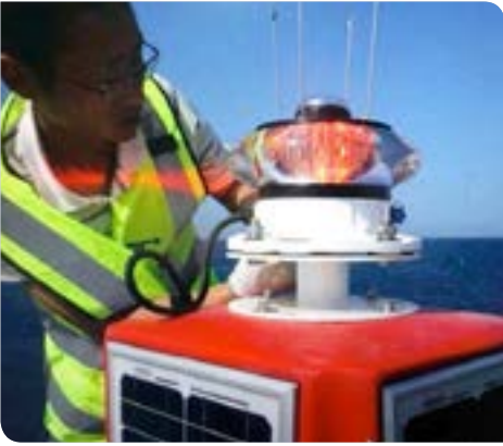
SL-155-2D5 Lantern, 2.5 degree lens enabling up to 14NM range from a self-contained SL-C600 solar system. Note the reflections from the narrow beam on the clothing of the technician.
