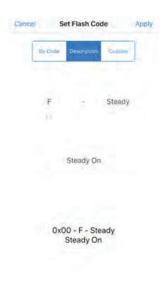
**2. Code** – Select the Flash Code from the Sealite Flash Code table provided in the Appendix section. Once the Flash Code is established press "Set / Apply" to confirm the change.
