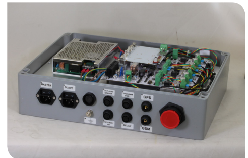
LED Controller with 110/240V supply
